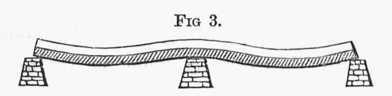
over the pivot does not attain its greatest intensity until both spans are fully loaded; it is then equal to the sum of the effects due to the dead load, which is carried wholly by the pivot pier, plus the effects of the live load, which is distributed according to the laws which govern a continuous beam resting on three supports. The moment due to the moving load, is at the centre the negative of that at the centre of one arm when loaded alone, being equal to
