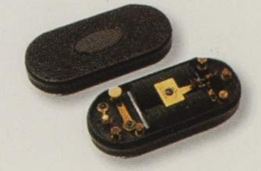
POCKET TELEGRAPH KEY USED IN KANSAS, 1861-1865.
