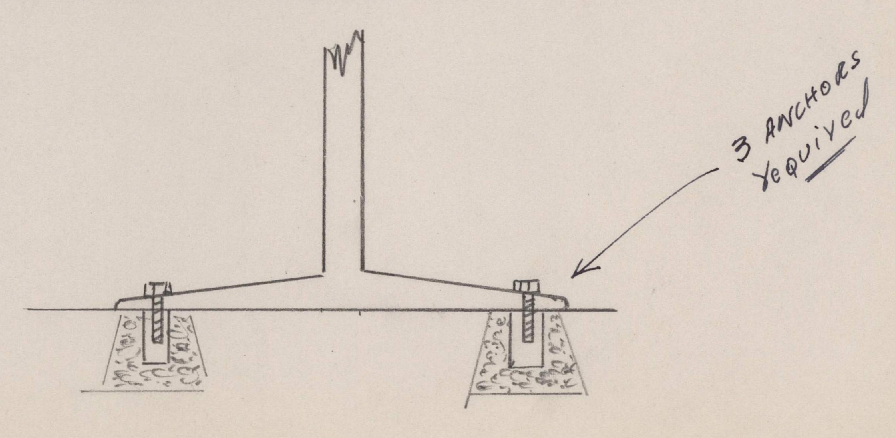
(B) Special movable type for use on concrete or other hard surface play yard. To consist of cup to be imbedded in concrete. Standard to fit in cup as illustrated.
