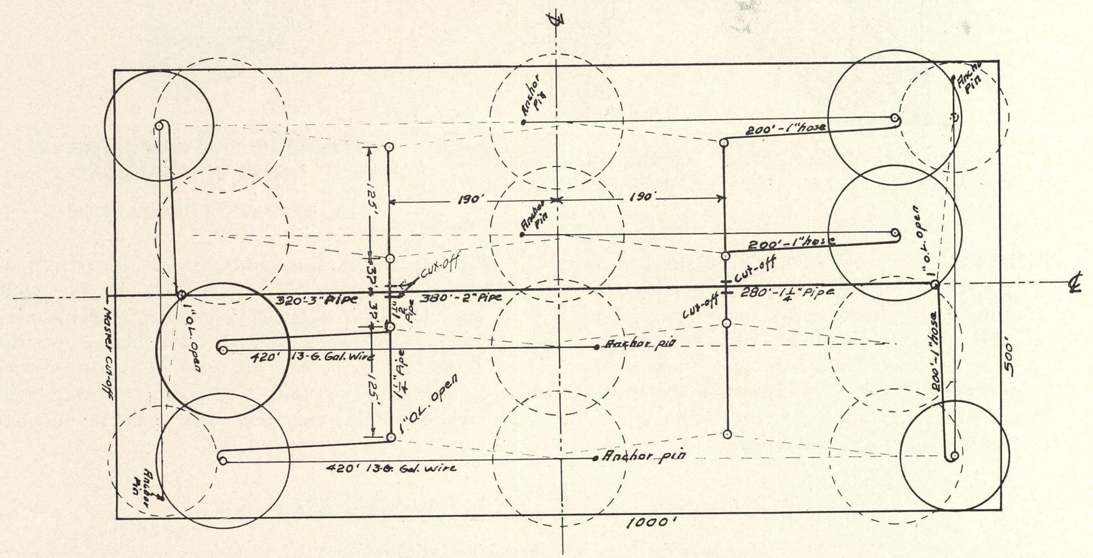
A practical and efficient layout for a full sized Polo Field, to be watered with Economy Traveling Base Units, showing location of outlets.
