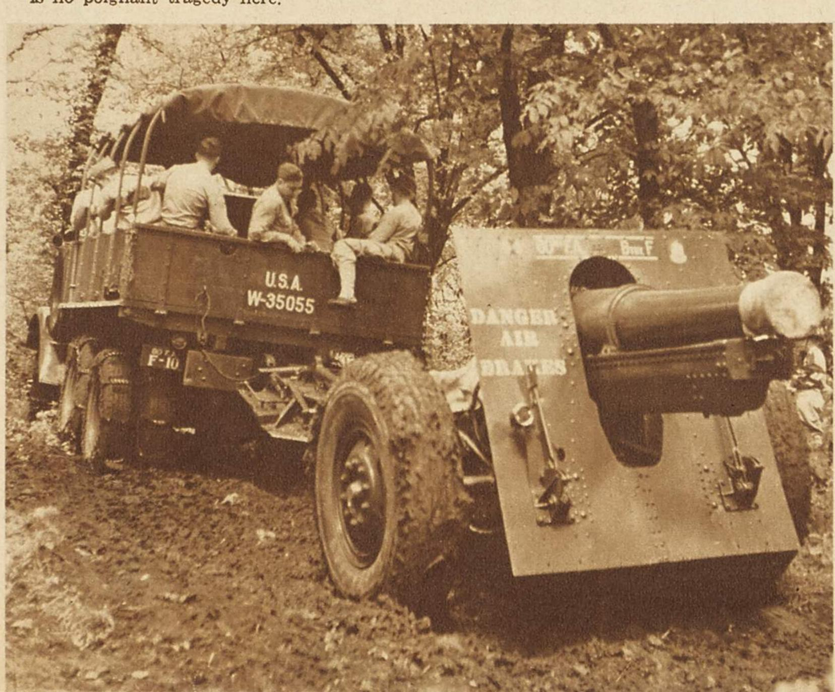
A BIG JOB FOR ANY TRUCK - This army truck is a stanch and powerful vehicle, as it needs must be for this task, pulling a 155-millimeter howitzer up a slick hill. All of the many wheels of the truck wear chains, but those of the howitzer aren't so equipped. The tube (or barrel) of the gun alone weighs 2,600 pounds.
