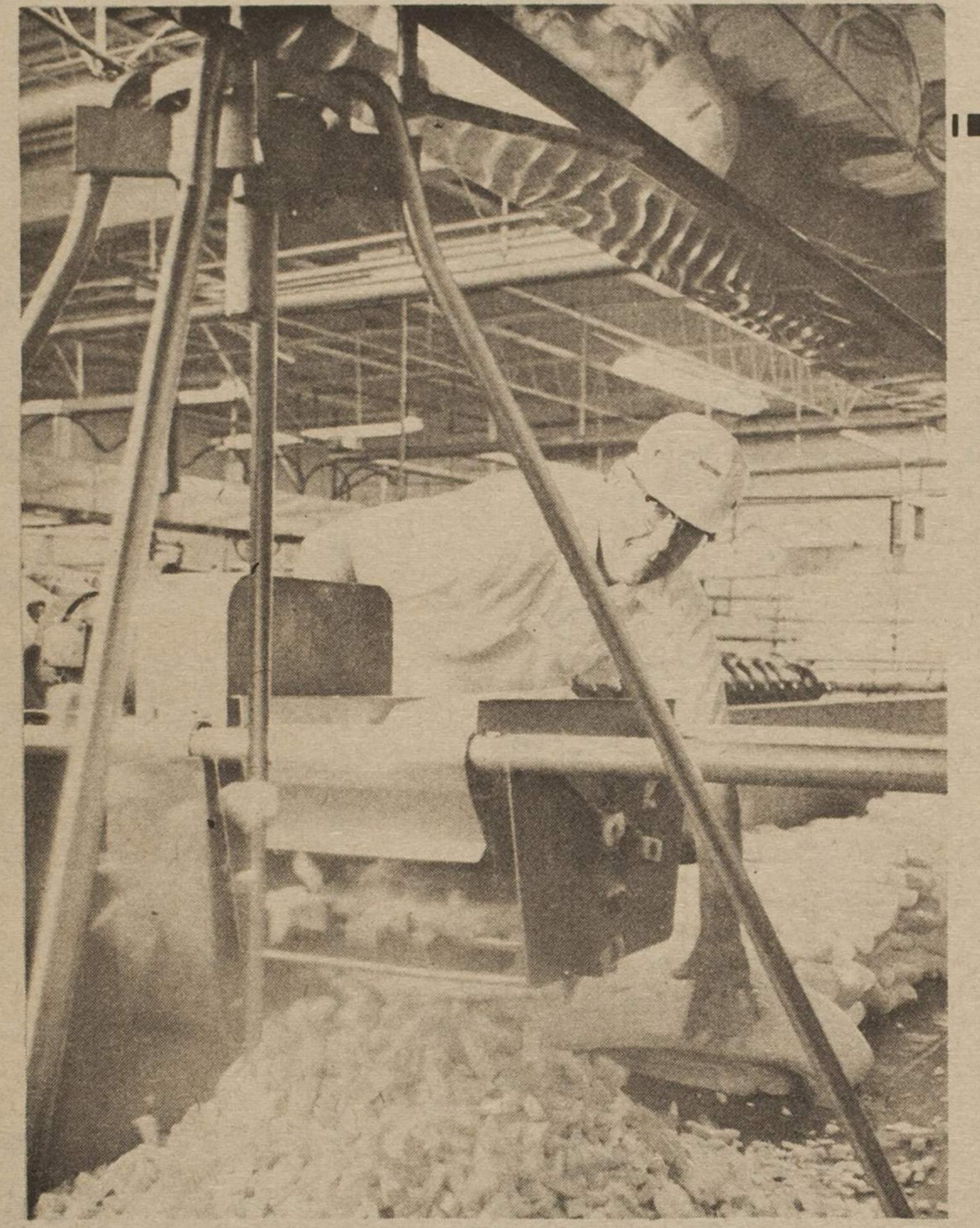
The slabs are fed into a machine which cuts them up into nibble-size pieces. And at this point in the process, they are already good enough to eat!
