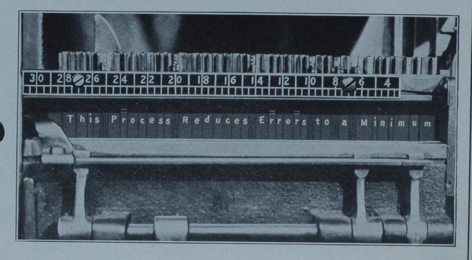
, in glancing at the assembler, your composing machine operators could read the mats before the line was cast
